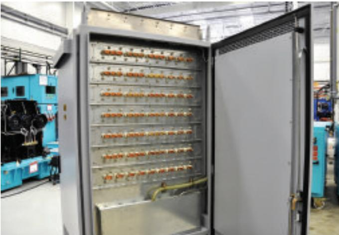
The TLB-R1000 load bank is UL Listed and utilizes Testek's proprietary resistor load elements constructed from precision nickel-chromium resistance alloy, which are fully supported within the air stream by stainless-steel rods that are insulated with high-temperature refractory ceramics.
