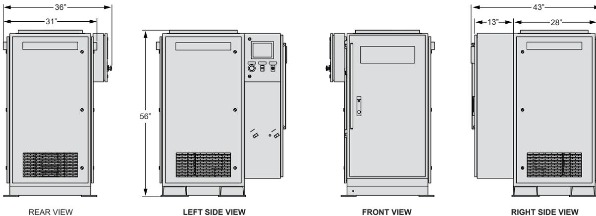
The load bank resistor elements are forced-air cooled with a heavy-duty, three-phase, TEFC electric blower motor with a high-performance direct-drive fan blade. The blower motor can be powered from the main input load bus (test source) or optionally from an external three-phase supply source. Motor starter circuit is fuse protected and includes an overload relay.
