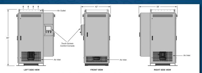
The load bank resistor elements are forced-air cooled with a heavy-duty, three-phase, TEFC electric blower motor with cast aluminum, highperformance direct-drive fan blade. The blower motor can be powered from the main input load bus (test source) or optionally from an external three-phase supply source. Motor starter circuit is fuse protected and includes an overload relay.
