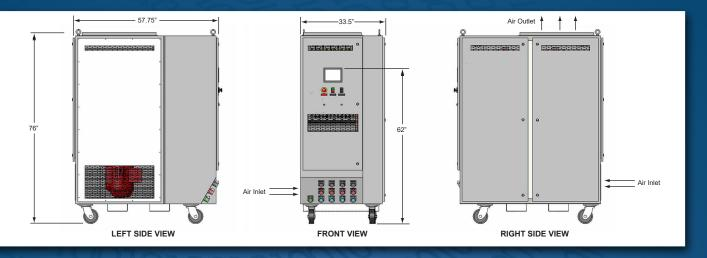
The load bank resistor elements are forced-air cooled with a heavy-duty, three-phase, dual-voltage blower motor with cast aluminum, highperformance direct-drive fan blade. The blower motor can be powered from the main input load cables (test source) or optionally from an external three-phase supply source. Motor starter circuit is fuse protected and includes an overload relay.
