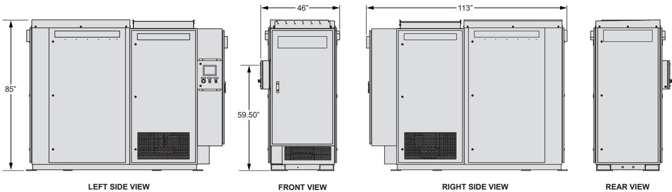
The load bank resistor elements are forced-air cooled with a heavy-duty, three-phase, TEFC electric blower motor with a high-performance direct-drive fan blade. The blower motor can be powered from the main input load bus (test source) or optionally from an external three-phase supply source. Motor starter circuit is fuse protected and includes an overload relay. The reactors have supplemental cooling by internal 120 VAC blowers powered from the main control circuit.
